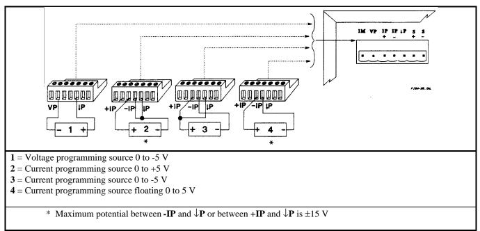
Figure 4-5g. Series 668xA Analog Programming Connections
